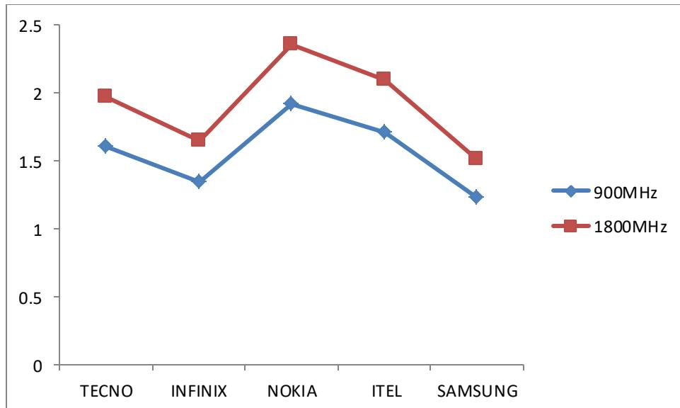
**Figure 1: Comparison of the average SAR values for various phone models operating at 900MHz and 1800MHz to ICNIRP reference levels/recommended limits.**
